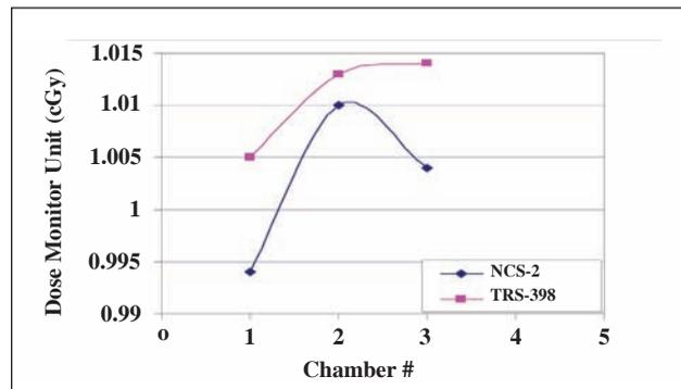
**Fig. 3:** Dose per monitor unit of the different ionization chambers in an 18 MV photon beam calculated with the two dosimetry protocols.
