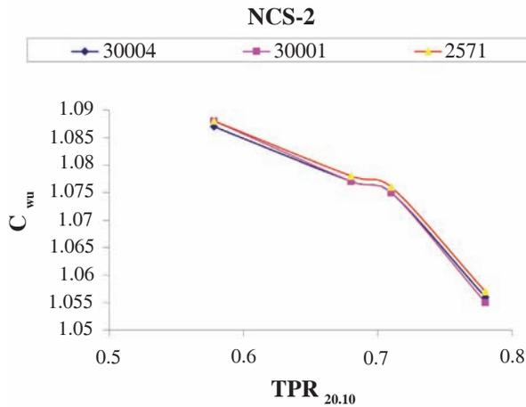
Fig. 1: Air kerma to absorbed dose to water overall conversion factors according to NCS Report-2.
