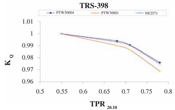
Fig. 2: The relation between  $TPR_{20,10}$  and Absorbed dose beam quality conversion factor  $K_Q$  According to IAEA TRS-398 protocol.
