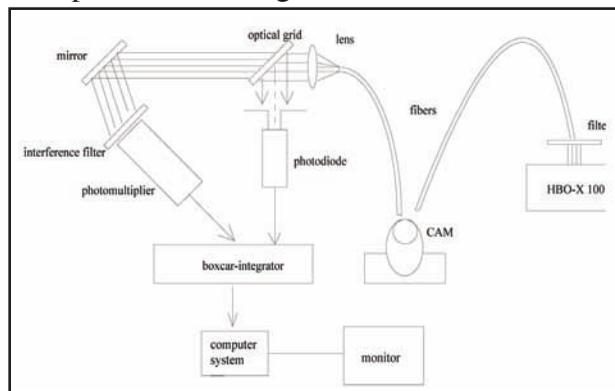
**Fig. 2: Experimental set-up of the fluorescence measurements**
